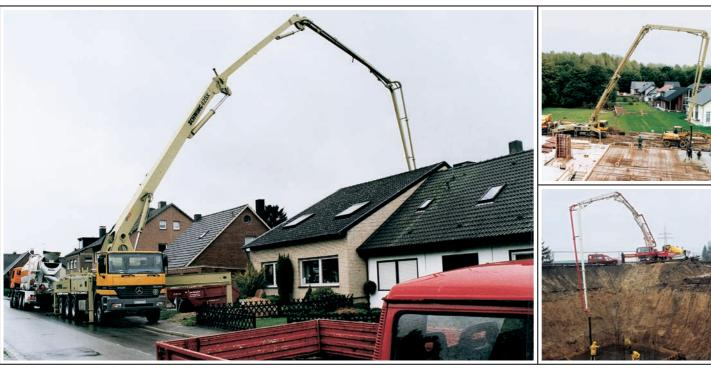
SCHWING **EASy** – our optional single-sided set-up for fail-safe operation when the pump can only be stabilized on one side. An abliability insurers (BIA). be stabilized on one side. An absolute must for machines that need
