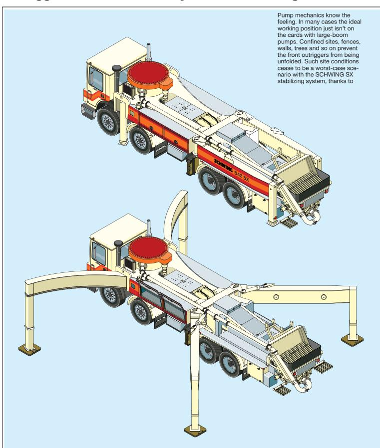
the telescoping front outriggers. This system not only makes for short set-up times but can also add decisively to the working range of the placing
